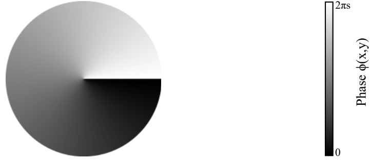
Figure 2.6: Azimuthally varying phase pattern to imprint a vortex with integer angular momentum s . The angular momentum s depends on the discontinuity equals 2\pi s . The color map represents the phase gradient.
