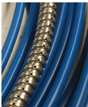
(b) Metal and plastic fiber protection hose. The metal hose is used within the vacuum and slotted for evacuation.
